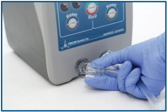
1) Open new tubing package(s). Attach time and date sticker directly to the tubing. Install air tubing set to either of the air output ports located on the lower front of the unit.
