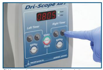
5) Use + or - buttons to adjust airflow cycle time if desired. Time shown in minutes.
