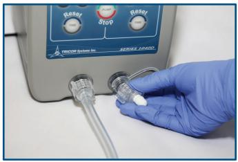
2) Install the included air output cap on the opposite port if only running one endoscope.
