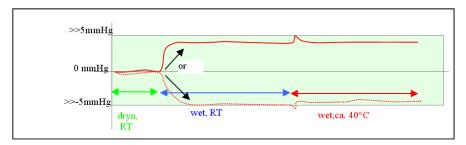
Typical curve of an unclean and crusted sensor
