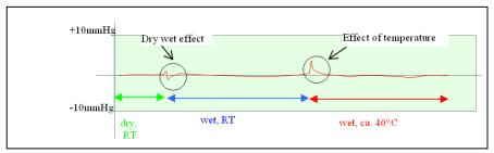
Typical curve of a clean sensor [Dry 20 °C / 68 °F  $\to$  Wet 20 °C / 68 °F  $\to$  Wet 40 °C / 104 °F]
